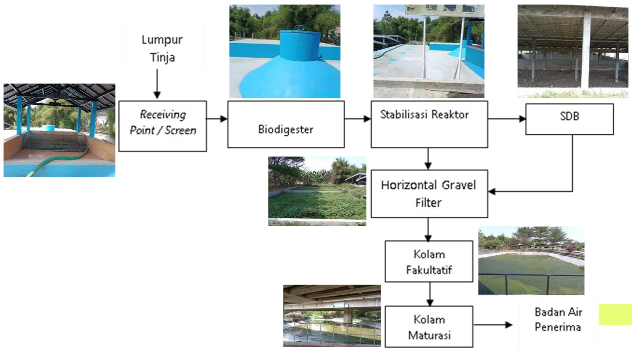
Gambar 2. 23 Diagram Proses IPLT Tegal Gundil Eksisting
